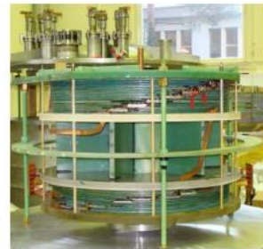
814 kJ Bi 2212 tape 315 A 20 K conduction cooled Diameter: 300/814 mm Height: 222 mm
