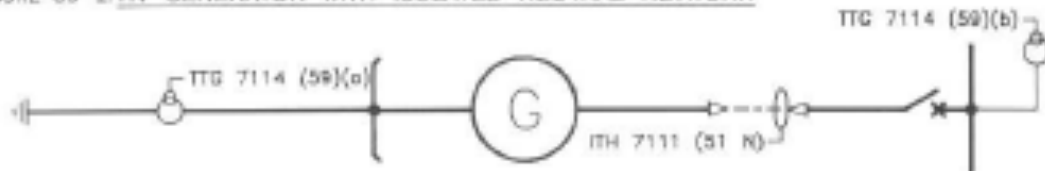
FIGURE C3-2: HV GENERATOR WITH ISOLATED NEUTRAL NETWORK
