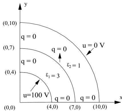
Figure 9. A quarter section of the coaxial cable that was divided in two subregions
