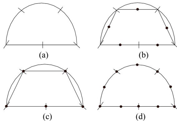
Figure 1. (a) Divided problem region, (b) Constant element, (c) Linear element, (d) Parabolic element
