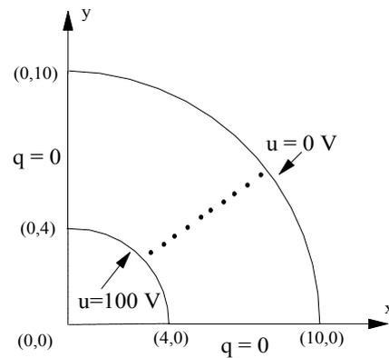
Figure 6. A quarter section of the coaxial cable
