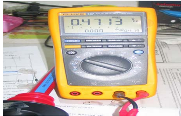
Figure 7 Experimental output voltage of doubler circuit
