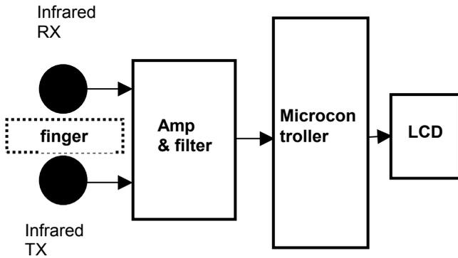
Figure 1. Block diagram of the measuring device
