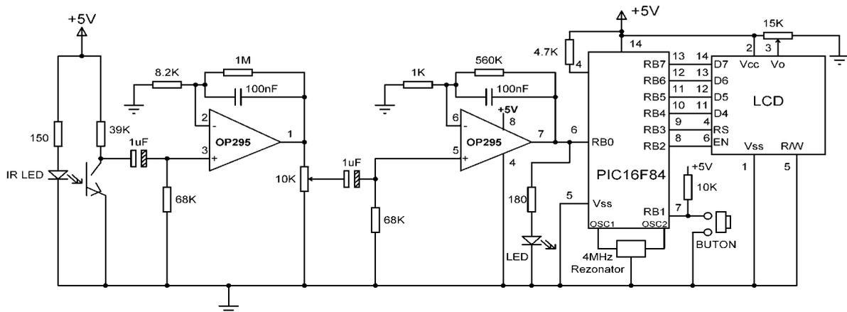
Figure 3. Circuit diagram of the device
