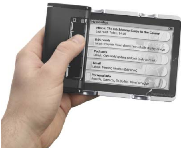
Fig. 8: Polymer Vision, a PDA with a folding screen. Here, the screen is unfolded unfolded [8].
