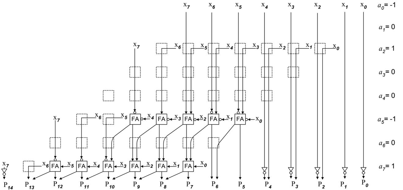
Figure 1. A parallel multiplier with eliminated the rows corresponding to the zero bits of the coefficient  $a = 10\bar{1}0010\bar{1}$ .
