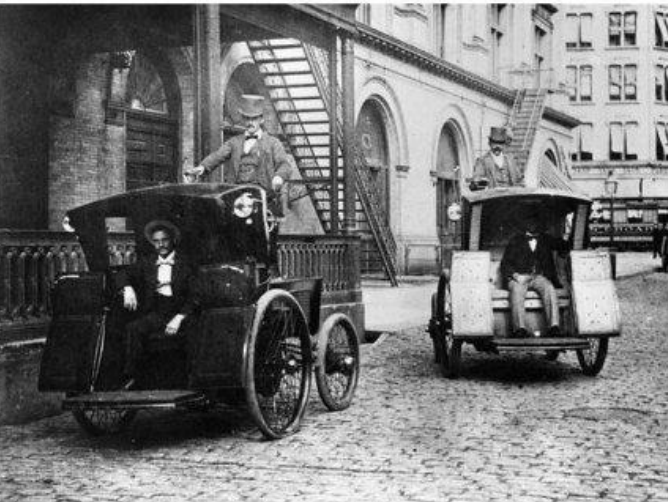
FIG. 30.—Front-Driving Brougham of the Electric Vehicle Co., used in New York City. This model, which is no longer manufactured, represents a construction very suitable for city service, but quite inappropriate for country and general use.
