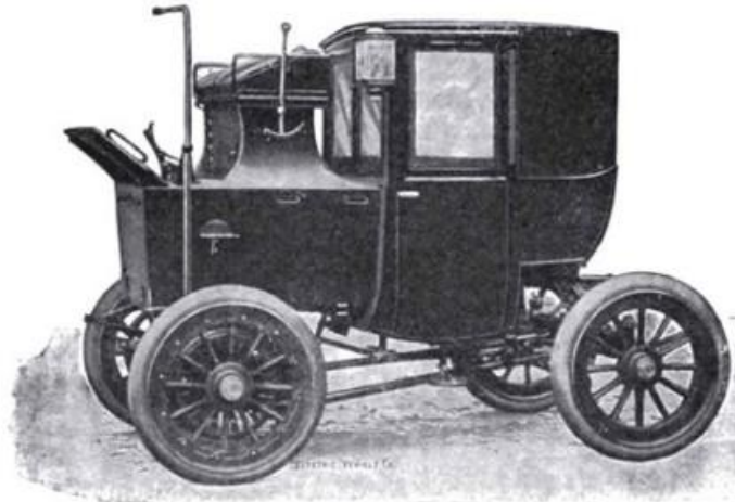
FIG. 30.—Front-Driving Brougham of the Electric Vehicle Co., used in New York City. This model, which is no longer manufactured, represents a construction very suitable for city service, but quite inappropriate for country and general use.
