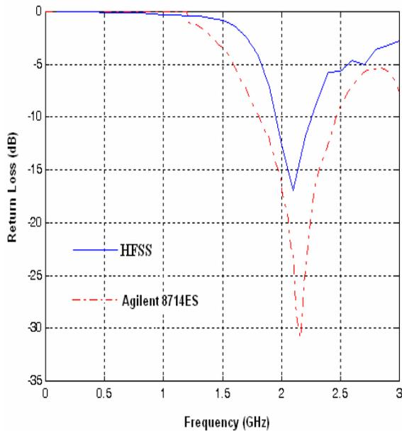
Figure 4.5. : The Return Loss (dB) Characteristics realised after the measurements and the simulations
