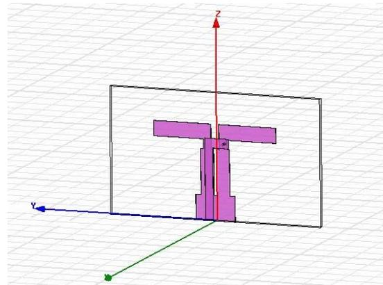
Figure 4.4. : HFSS Printed Dipole Antenna Model
