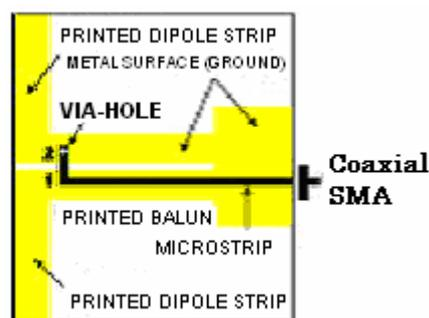
Figure 2.1. : Printed Dipole Antenna with Microstrip Balun [3]
