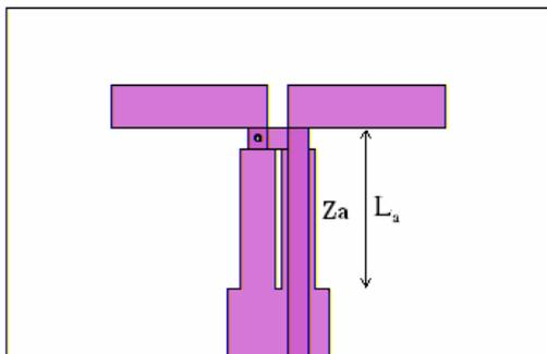
Figure 2.4. : Printed Dipole Antenna
