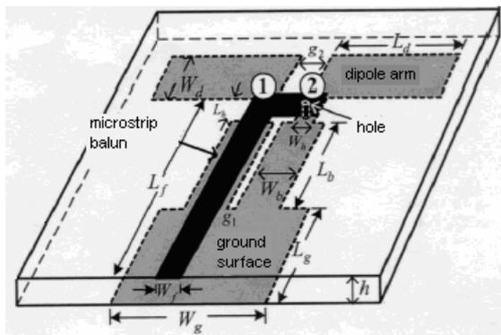
Figure 4.1. : The geometry of the Printed Dipole Antenna[3]
