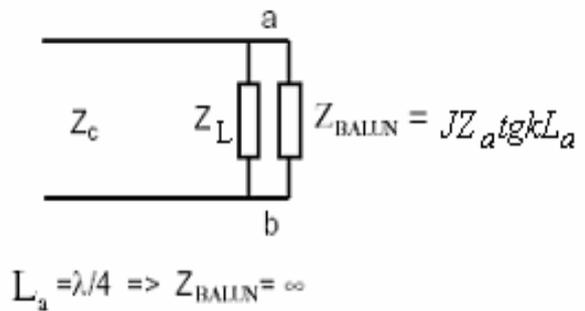
Figure 2.6. : Circuit Equivalent of The Printed Dipole Antenna
