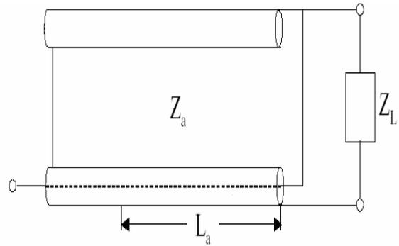
Figure 2.5. : Co-axial Equivalent of The Printed Dipole Antenna
