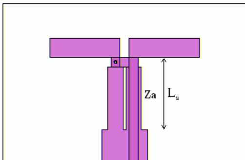
Figure 2.4. : Printed Dipole Antenna
