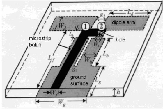
Figure 2.7. : The geometry of The Printed Dipole Antenna [3]
