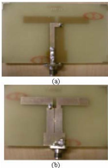
Figure 4.2. : 2.1 GHz Microstrip Printed Dipole Antenna
