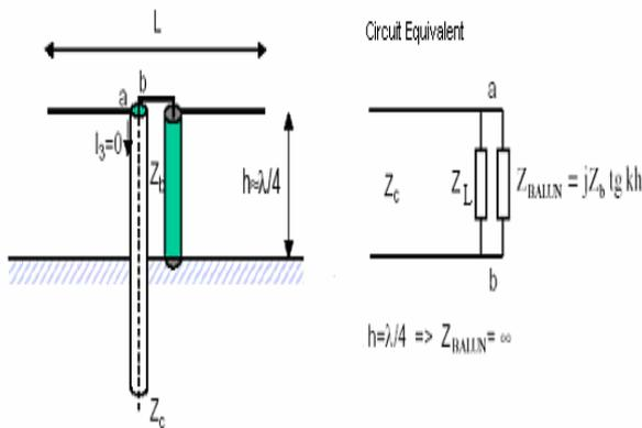
Figure 2.3. : Circuit Equivalent of Balun[4]
