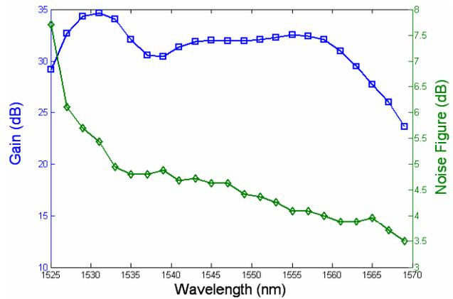
Figure 7. Gain and noise figure spectra of a 6 m long C band EDFA.  $P_{pump\ in} = 92.5\ mW$  and  $P_{sig\ in} = -30\ dBm$ .
