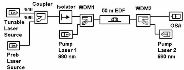
Figure 4. Bidirectionally pumped L band EDFA.
