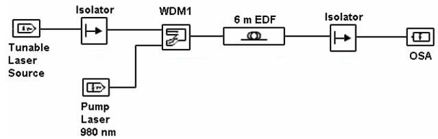
Figure 3. Forward pumped C band EDFA.
