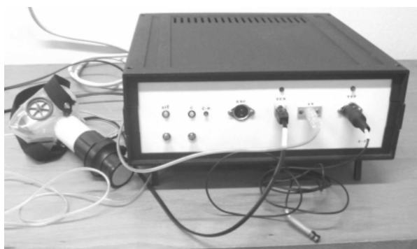
Figure 8. The KARD system with mask, ventilation and heart rate sensor and gas analyzer. KARD box size: 300 x 270 x 110 mm, weight: 2.2 kg.
