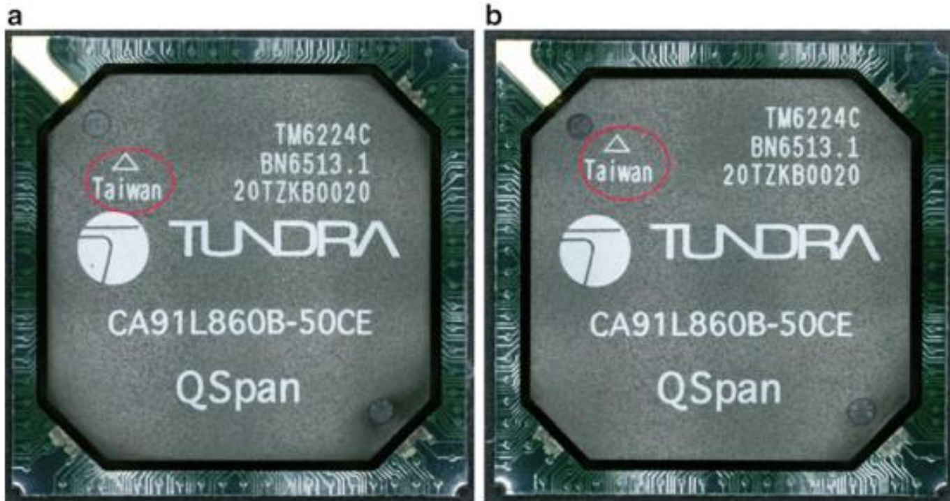
Fig. 3.16 Marking defects (a) Encircled marking near Tundra logo (b) Encircled marking near mold mark
