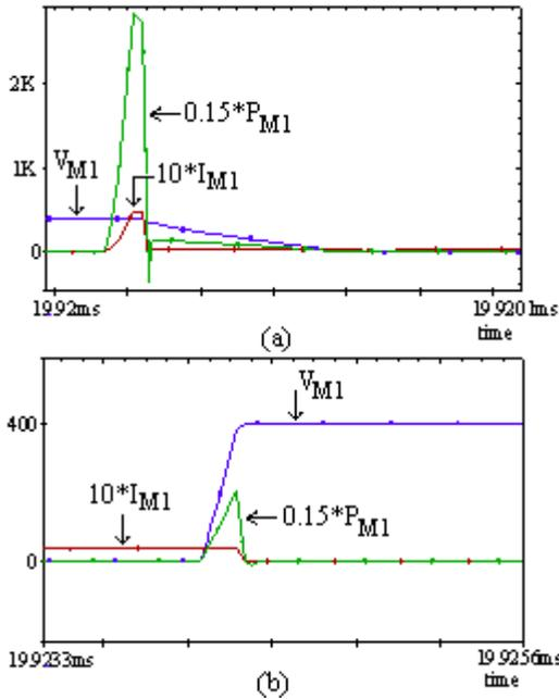
**Fig. 4.** Spice simulation results of the hard-switched two-leg interleaved boost topology, (a) for ON-time (b) for OFF-time (Green is Power loss) [Avg (PM<sub>1</sub>+PM<sub>2</sub>)=32W]
