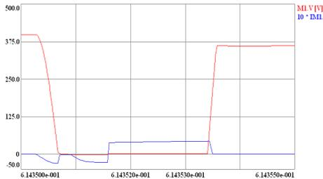
Fig. 9. Simplorer simulation result of main switch (M1) voltage-current waveforms
