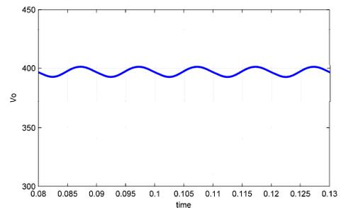
**Fig. 6.** Simplorer simulation result of output voltage (400V)
