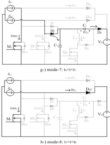
**Fig. 3.** The equivalent circuits of the operating modes (for  $D > 0.5$ ) in one switching cycle
