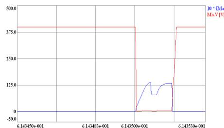
Fig. 10. Simplorer simulation result of auxiliary switch (Ma) voltage-current waveforms
