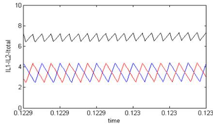
Fig. 8. Simplorer simulation result of inductors' current and total current waveforms
