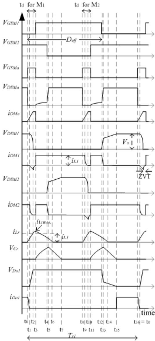
Fig. 2. Operating waveforms of the proposed converter for one switching cycle (for  $D > 0.5$ )
