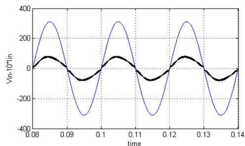
**Fig. 7.** Simplorer simulation result of input voltage-current (V<sub>inrms</sub>=220V; I<sub>inrms</sub>=4.63A) waveforms ; (pf=0.989, THD=8%)
