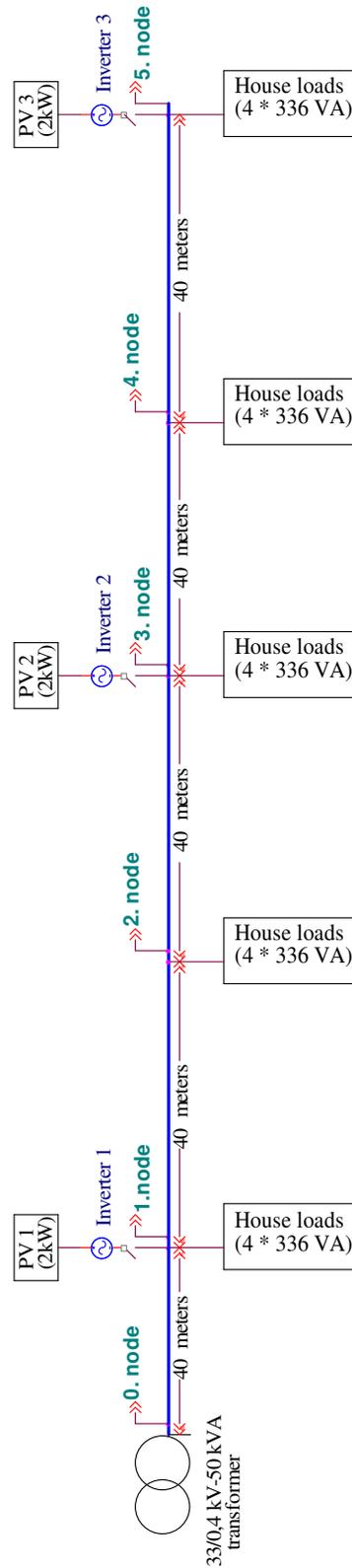
Figure 2 Single line scheme of the modelled system.
