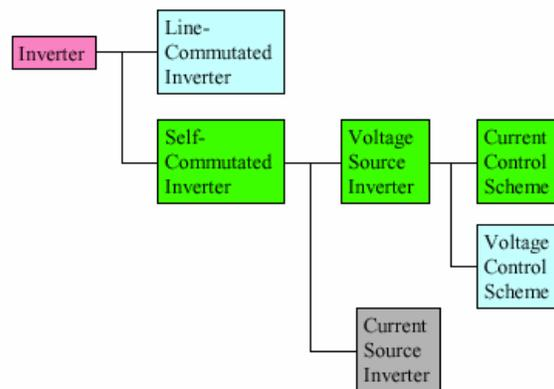
Figure 1 Classification of inverter types.
