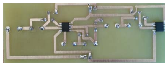
Fig. 9. Pcb design of Butterworth low pass filter
