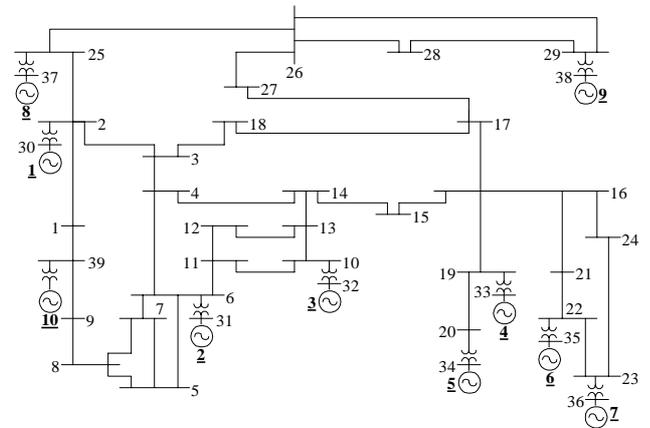
Figure – 3.1 New England test system
