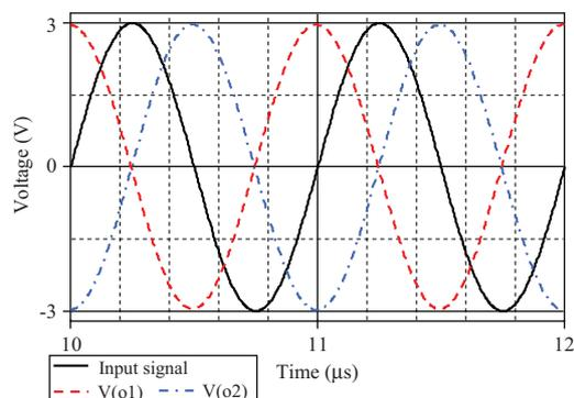
**Fig. 6.** Time-domain response of the proposed all-pass filter at 1 MHz
