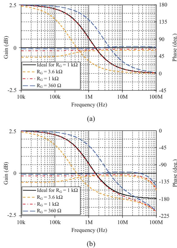
**Fig. 5.** Electrical tunability of the pole frequency by the degenerating resistor  $R_G$ : (a) inverting, (b) non-inverting VM first-order all-pass filter responses
