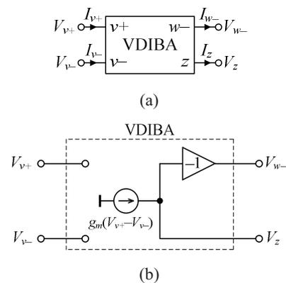
Fig. 1. (a) Circuit symbol, (b) behavioral model of VDIBA
