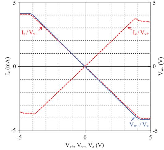
**Fig. 4.** DC analysis of VDIBA in Fig. 3:  $I_z$  versus  $V_{v+}$  and  $V_{v-}$ ,  $V_{w-}$  versus  $V_z$
