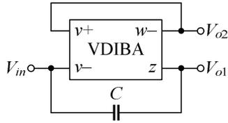
**Fig. 2.** Proposed resistorless dual-output VM all-pass filter with electronic tuning
