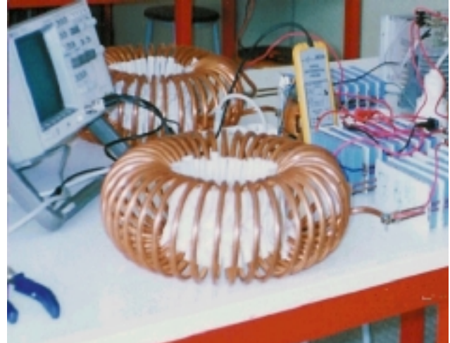
Fig. 4. A Toroidal Shaped Cylindrical Form Air-Core Inductor Design Capable of Operating at 20 kHz, 500 V pk and 200 A pk .
