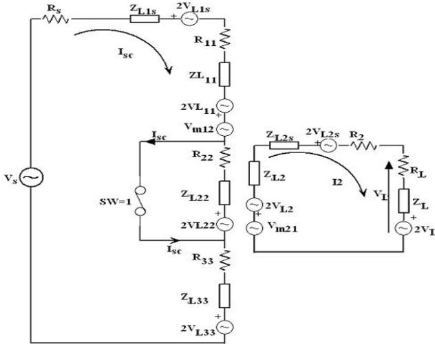
Figure 7. A Turn to turn fault at primary side (a TLM example).
