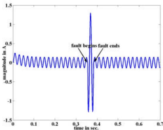
Figure 8. Primary current of the transformer during internal short circuit in wavelet based modeling
