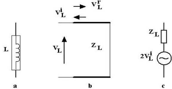
Figure 3. a) inductance, b) stub model of inductance, c) TLM equivalent circuit
