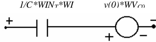
Figure 4. Transient model of a capacitance in wavelet domain [12], [13].
