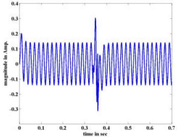
Figure 9. Primary current of the transformer during internal short circuit in TLM based modeling
