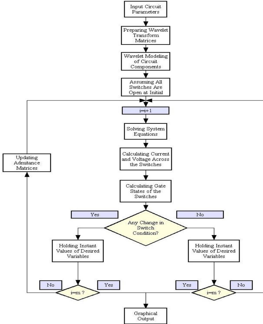
Figure 6. The proposed simulation algorithm
