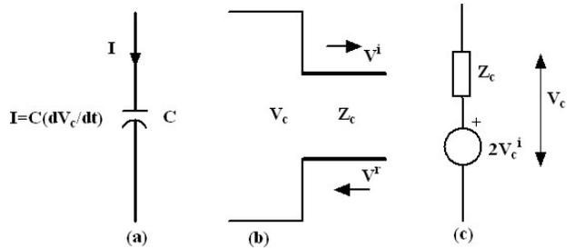
Figure 5. A capacitance, (a) in time domain, (b) its TLM representation, and (c) its Thevenin equivalent.
