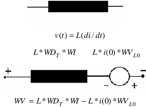
Figure 2. Transient model of inductor in wavelet domain [12], [13]
