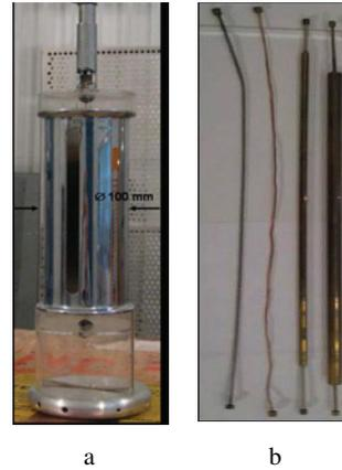
Fig. 2. a) Coaxial electrode system; b) Wire electrodes.
