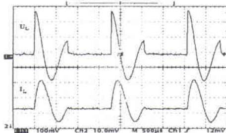
Figure 5 Measured load voltage v_L and load current i_L [CH1:100V, CH2:20A, T:0.5mS].
