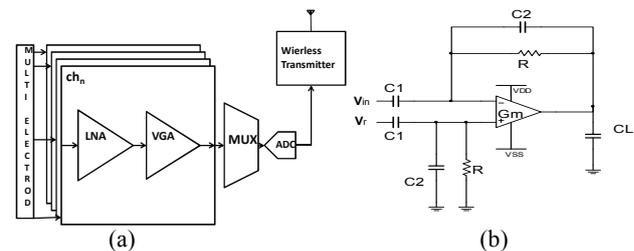
**Fig. 1.** (a) Structure of a system for recording neural signals; b) An amplifier of neural signals [5]
