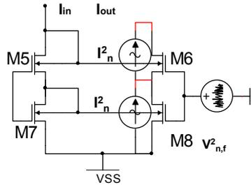
Fig. 3. Sources of noise in BDCCM circuit
