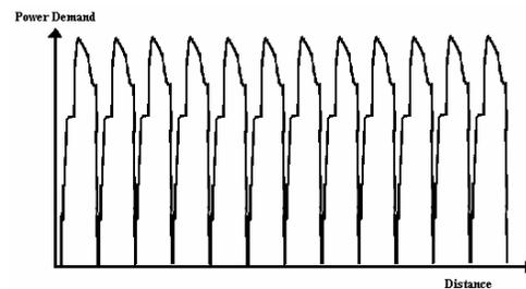
Fig. 3. Power demand characteristics of the Tabriz urban railway train sets from the first station to the last.
