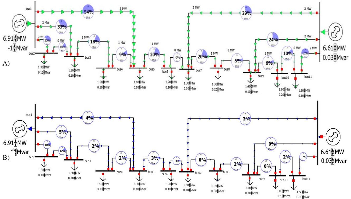
Fig. 4. Power load flow analysis of the AC distribution system, A)active power, B)reactive power.
