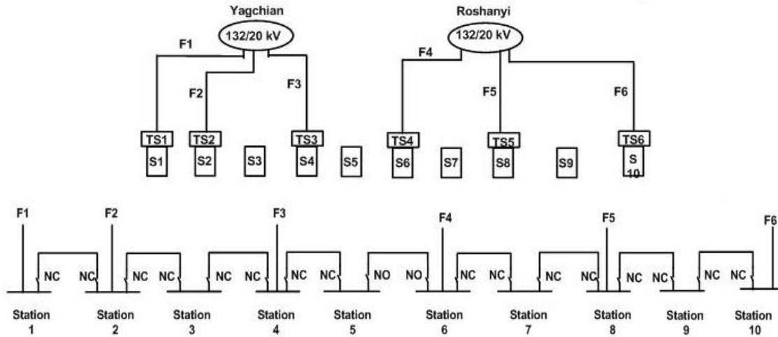
Fig. 1. Single line diagram of power distribution system for Tabriz urban
