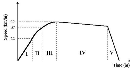
Fig. 2. Speed characteristics of the train sets with time and place variations.
