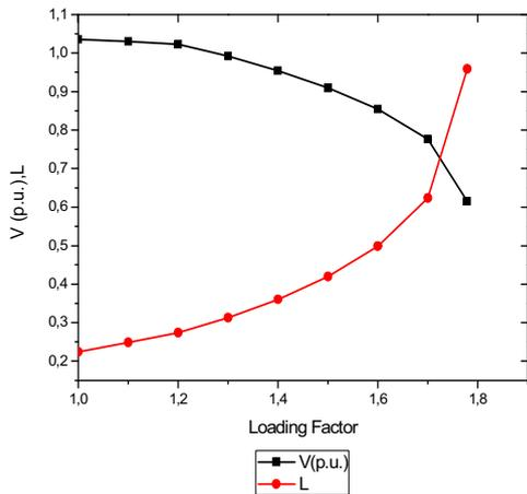
**Fig. 3** Stability indicator L and its relation to the critical voltage of IEEE 14 busbar test system
