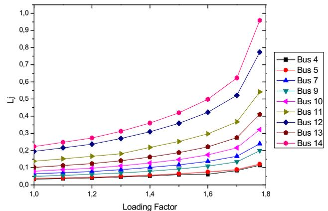
Fig. 2 Evaluation of  $L_j$  index versus load variation for IEEE 14 busbar test system
