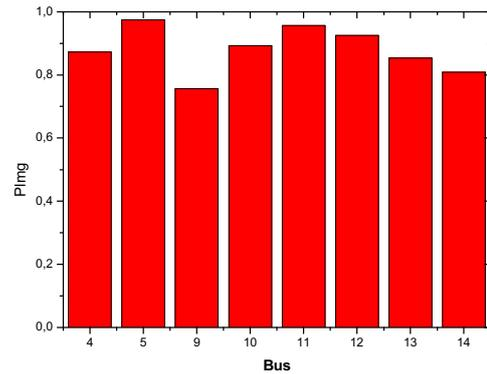
Fig. 1 Local load margin index for IEEE 14 busbar test system
