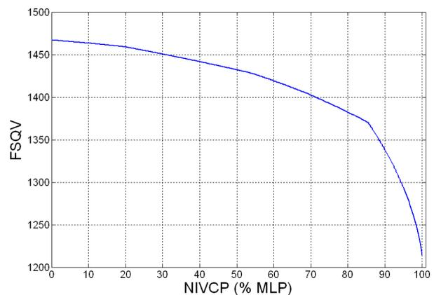
**Fig. 9** – NIVCP curve for IEEE 57 bus system
