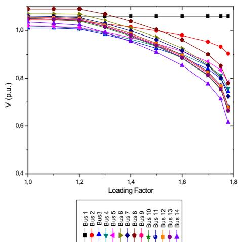
**Fig. 4** P-V Curves for IEEE 14 busbar test system
