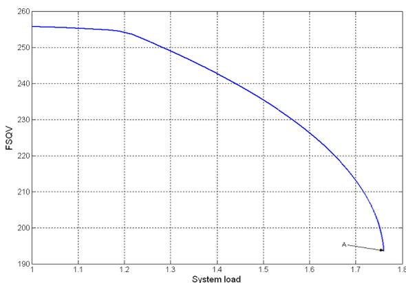
**Fig. 7** FSQV curve for IEEE 14 bus system
