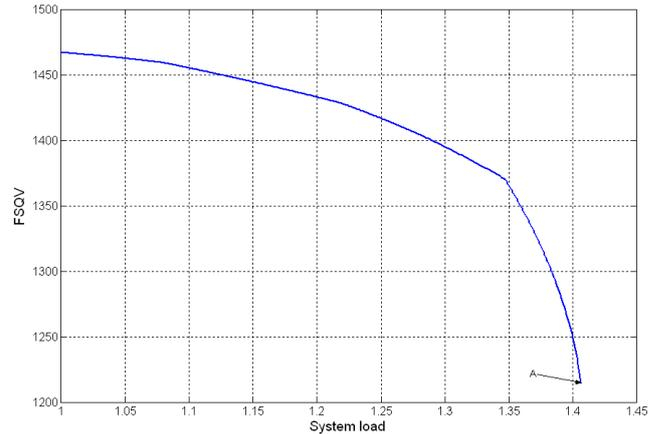
**Fig. 8** FSQV curve for IEEE 57 bus system
