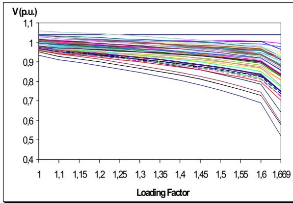
**Fig. 6** P-V Curves for IEEE 57 busbar test system
