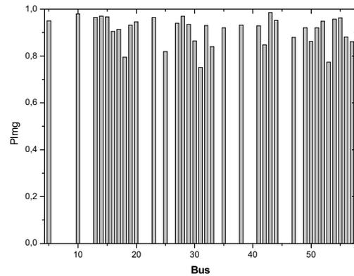
**Fig. 5** Local load margin index for IEEE 57 busbar test system
