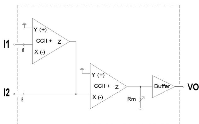
Figure 3: CCII+ based variable-Rm OTRA topology
