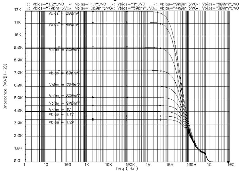
Figure 8: Typical ac simulation result, transresistance of the CMOS variable-Rm OTRA with  $V_{bias} = 0.3 \text{ V} - 1.2 \text{ V}$
