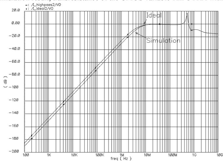
Figure 9: High-pass filter characterization of the ideal and the simulated CMOS OTRA with a typical ac simulation
