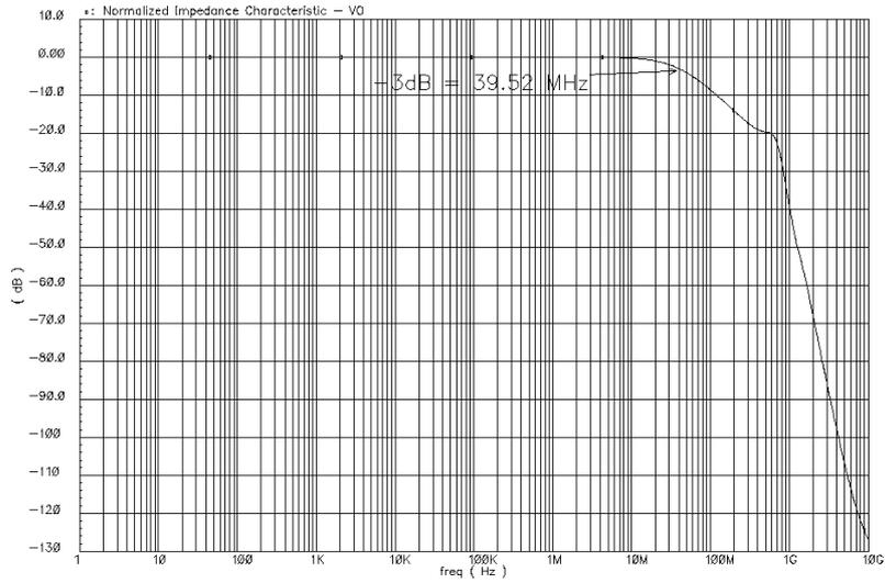
Figure 7: Typical ac simulation result, transresistance gain of the OTRA in a normalized axis with  $V_{bias} = 0.6 \text{ V}$
