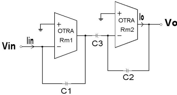
Figure 4: Proposed OTRA Rm-C high-pass filter
