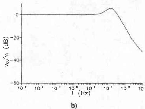
Fig.2. Device characteristics of the operational amplifier a) dc voltage transfer characteristic b) The unity gain frequency response of the output voltage
