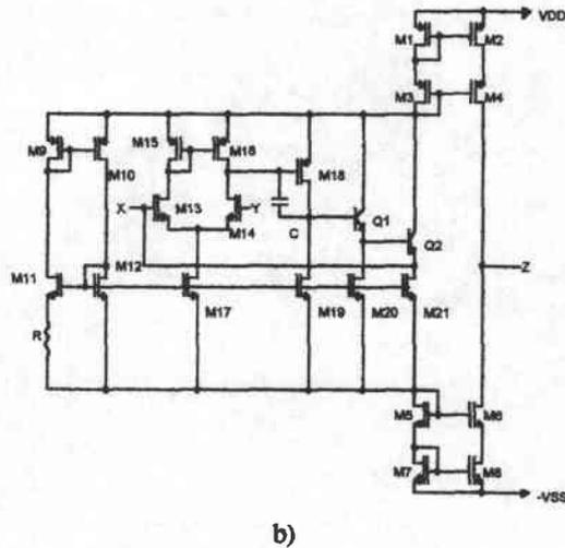
Fig.1. a) Current conveyor configuration b) Circuit diagram of the operational amplifier
