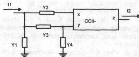
Fig.4. The bandpass filter configuration
