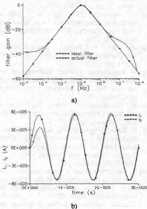
Fig.5. a) The frequency response of the filter b) The large-signal behavior of the filter
