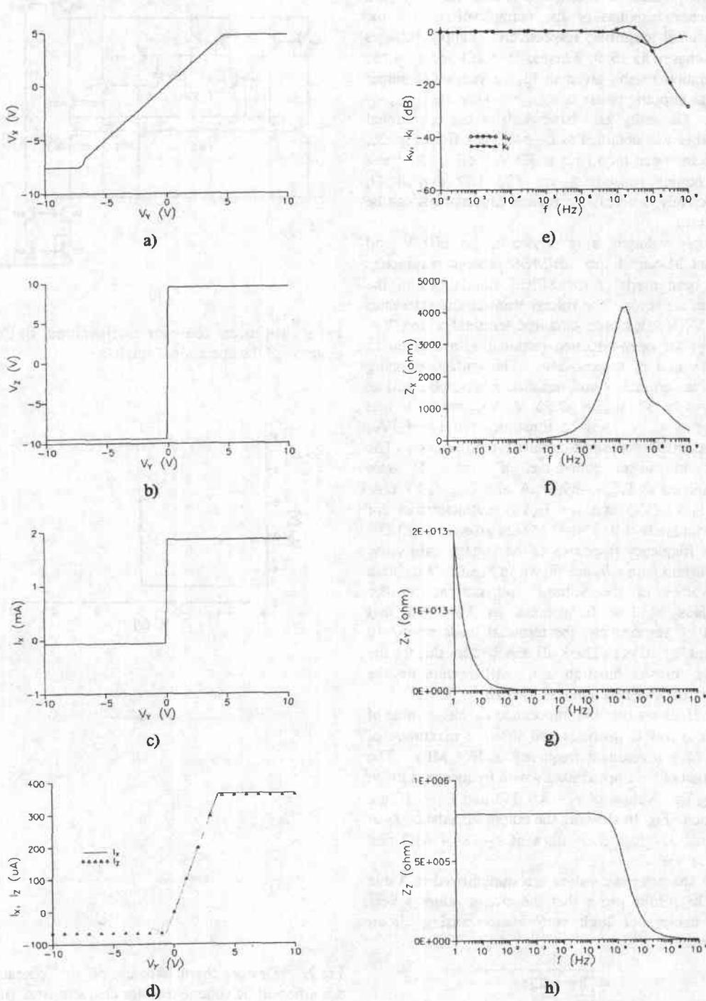
Fig.3. Device characteristics of the current conveyor a)  $V_x=V_x(V_y)$  for  $R_x=\infty$  b)  $V_z=V_z(V_y)$  for  $R_z=\infty$  c)  $I_x=I_x(V_y)$  for  $R_x=0$  d)  $I_x=I_x(V_y), I_z=I_z(V_y)$  for  $R_x=R_z=1 \text{ k}\Omega$  e) Frequency responses of  $v_x/v_y$  and  $i_z/i_x$  for  $R_x=R_z=10 \text{ k}\Omega$  f) Frequency response of  $Z_x$  g) Frequency response of  $Z_y$  h) The frequency response of  $Z_z$
