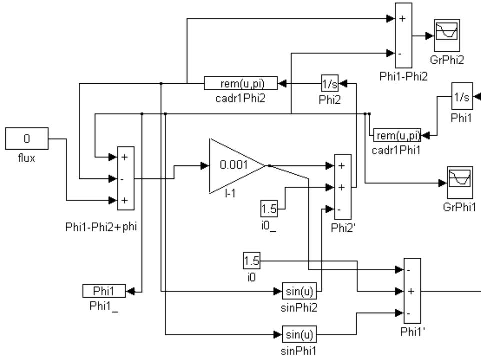
Fig. 2. MATLAB block diagram used to simulate a SQUID with low coupling
