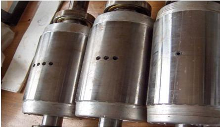
Fig. 5. Breaking of the rotor bars.
