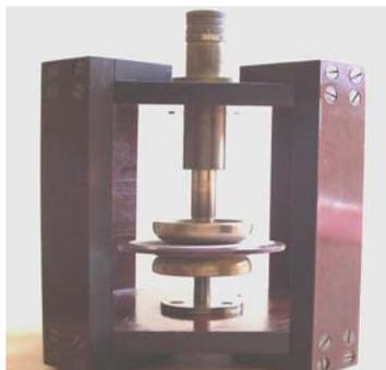
Figure 3. Rogowski electrode profile and a test sample
