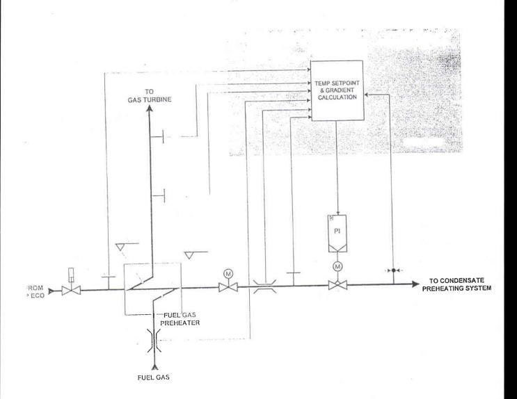
Fig. 1 Fuel Gas Preheater System
