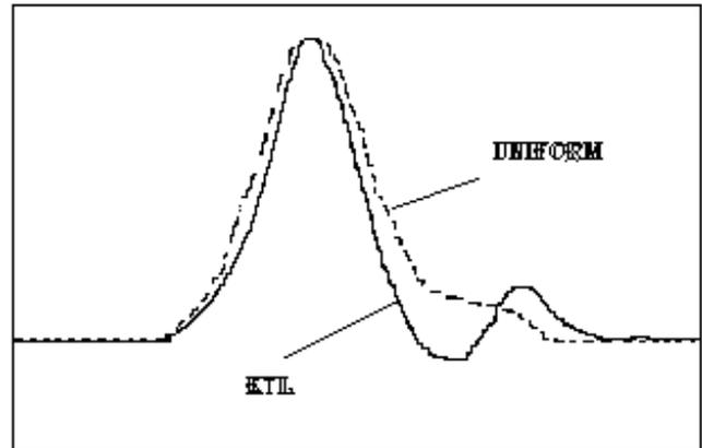
**Figure 3.** Difference in time response of PIN photodiode when coupled to ETL(solid) and when coupled to uniform transmission line (dashed).
