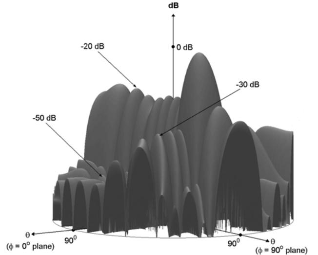
Figure 3. Three-dimensional pattern of the proposed planar array for  $L = 15$ ,  $d = 0.5\lambda$ ,  $\theta_0 = 35^\circ$ ,  $\phi_0 = 90^\circ$ ,  $R_v = 10^{3/2}$ ,  $R_u = 10$ ,  $BW_v = 35^\circ$  and  $BW_u = 30^\circ$
