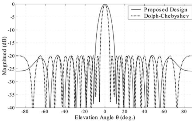
Figure 2. Patterns in the cross section  $\phi = 90^\circ$  ( $L = 17$ ,  $\theta_0 = \phi_0 = 0^\circ$ ,  $d = 0.5\lambda$ ,  $R_u = 10$ , and  $BW_v = 20^\circ$ )
