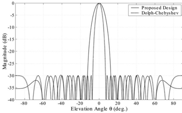
Figure 1. Patterns in the cross section  $\phi = 0^\circ$  ( $L = 17$ ,  $\theta_0 = \phi_0 = 0^\circ$ ,  $d = 0.5\lambda$ ,  $R_v = 10^{3/2}$ , and  $BW_v = 25^\circ$ )
