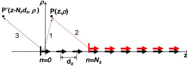
Figure 5. One-dimensional semi-infinite array and the application of synthetic aperture approach.
