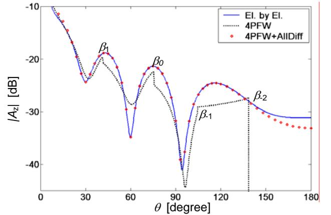
Figure 4. Amplitude of  $A_z$  vs.  $\theta$  radiated by a semi-infinite line array.
