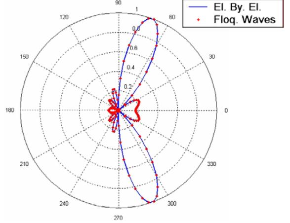
Figure 6. Amplitude of  $A_z$  versus  $\theta$  radiated by a rectangular array.
