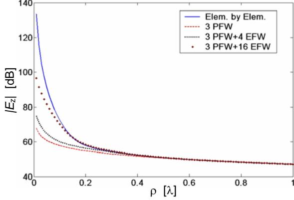
Figure 3. Amplitude of  $E_z$  versus  $\rho$  at  $z=0$  radiated by an infinite line array.
