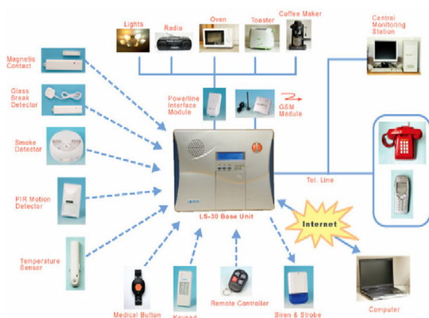
Figure 1. A sample home automation system
