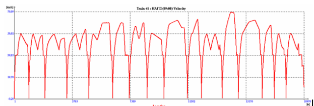
Figure 6. Speed vs. Location Profile for a train with the first coasting scheme
