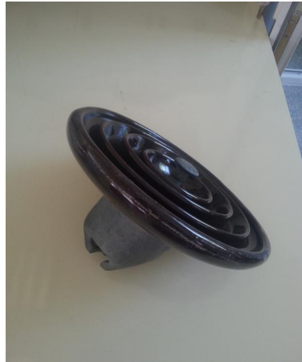
Figure 4. Photograph of U160 BL Insulator
