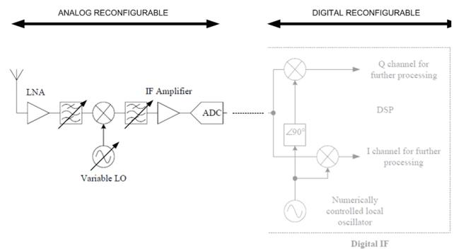
Fig. 4: Super-heterodyne structure with “digital IF” and reconfigurable narrowband elements.
