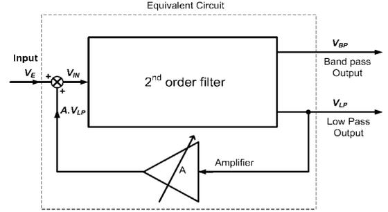
Fig. 10: Class 1 frequency agile filter made from the basic cell.
