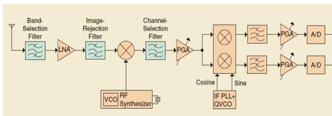
Fig. 1: Superheterodyne receiver architecture, [1].
