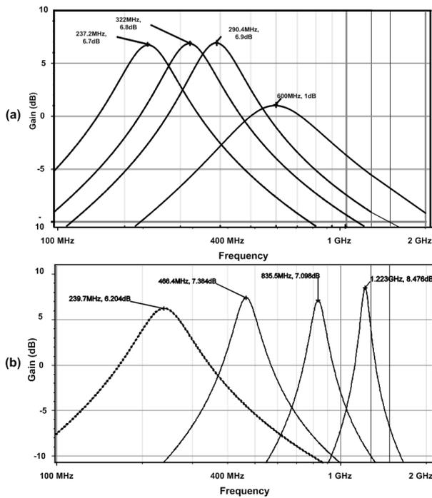
Fig. 16 : Frequency response of the frequency-agile filter.
