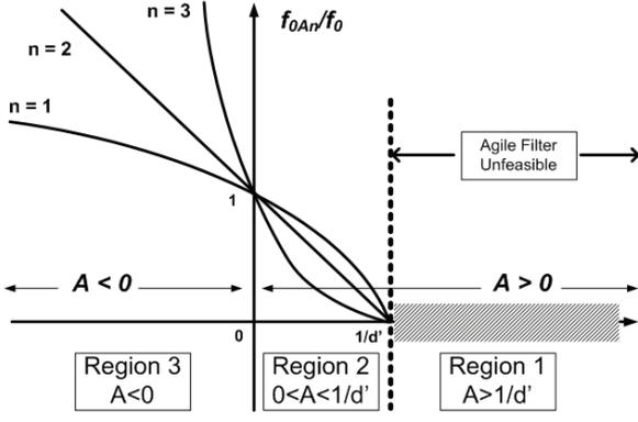
Fig. 12: Variation of  $f_{0An}/f_0$  as a function of gain  $A$  for various values of  $n$ .
