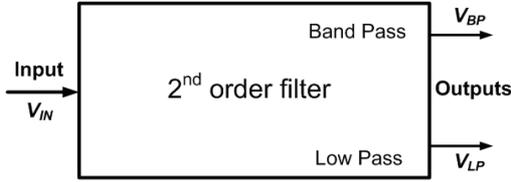
Fig. 9: Basic second order filter including two different outputs (class 0 agile filter).
