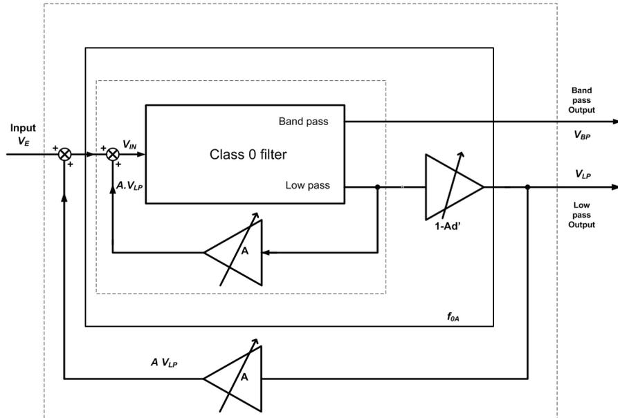
Fig. 13: Schematic implementation of the class 2 frequency agile filter.
