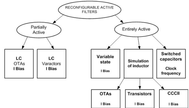
Fig. 6 : Classification of the reconfigurable active filters, [10-11].
