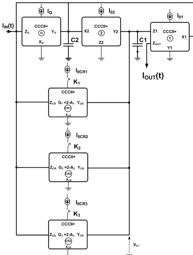
Fig. 15: Current-mode Frequency-agile filter with  $A < 0$ .
