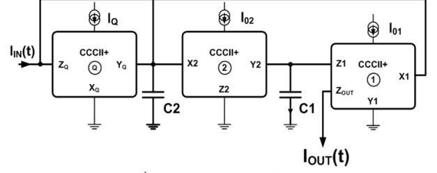
Fig. 14 : Zero-class 2<sup>nd</sup> order current mode filter.
