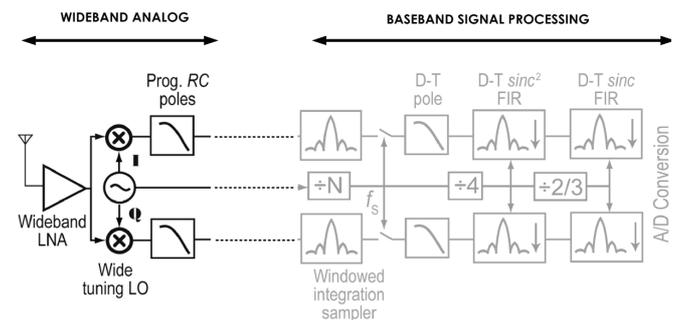
Fig. 3: Example of “zero IF” architecture with wideband reconfigurable elements
