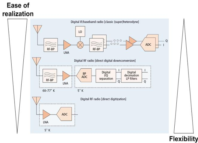
Fig. 5: flexibility versus the ease of realization of various architectures of multichannel reception, [10].
