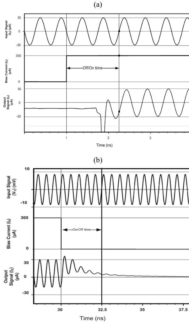
Fig. 8: Transient responses of the CCCII (a) "Off/On time",  $I_0$  varies from 0  $\mu\text{A}$  to 300  $\mu\text{A}$ ; (b) "On/Off time",  $I_0$  varies from 300  $\mu\text{A}$  to 0  $\mu\text{A}$ .
