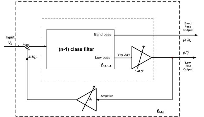
Fig. 11: Class  $n$  frequency agile filter.
