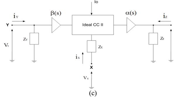
Fig. 7 : Current controlled conveyer CCCII+ :
