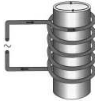
Figure 1: A workpiece in coil, the coil is energized from an AC source.
