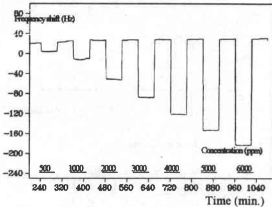
Figure 4.0 An example frequency shift (Hz) vs. concentration (ppm) at room temperature for our measurements
