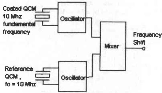
Figure 3. Block diagram of frequency shift measurement circuit
