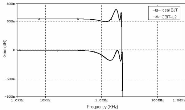
Figure 3. Maximum 0.177 dB passband ripple
