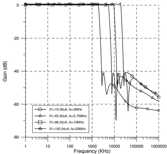
Figure 4. Tuning characteristics of the proposed filter
