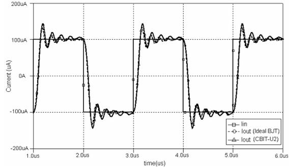
Figure 5. Step response of the filter
