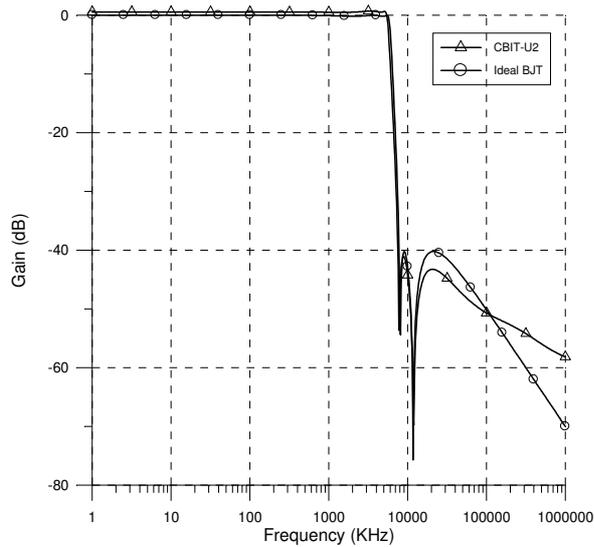
Figure 2. Gain response of the proposed filter
