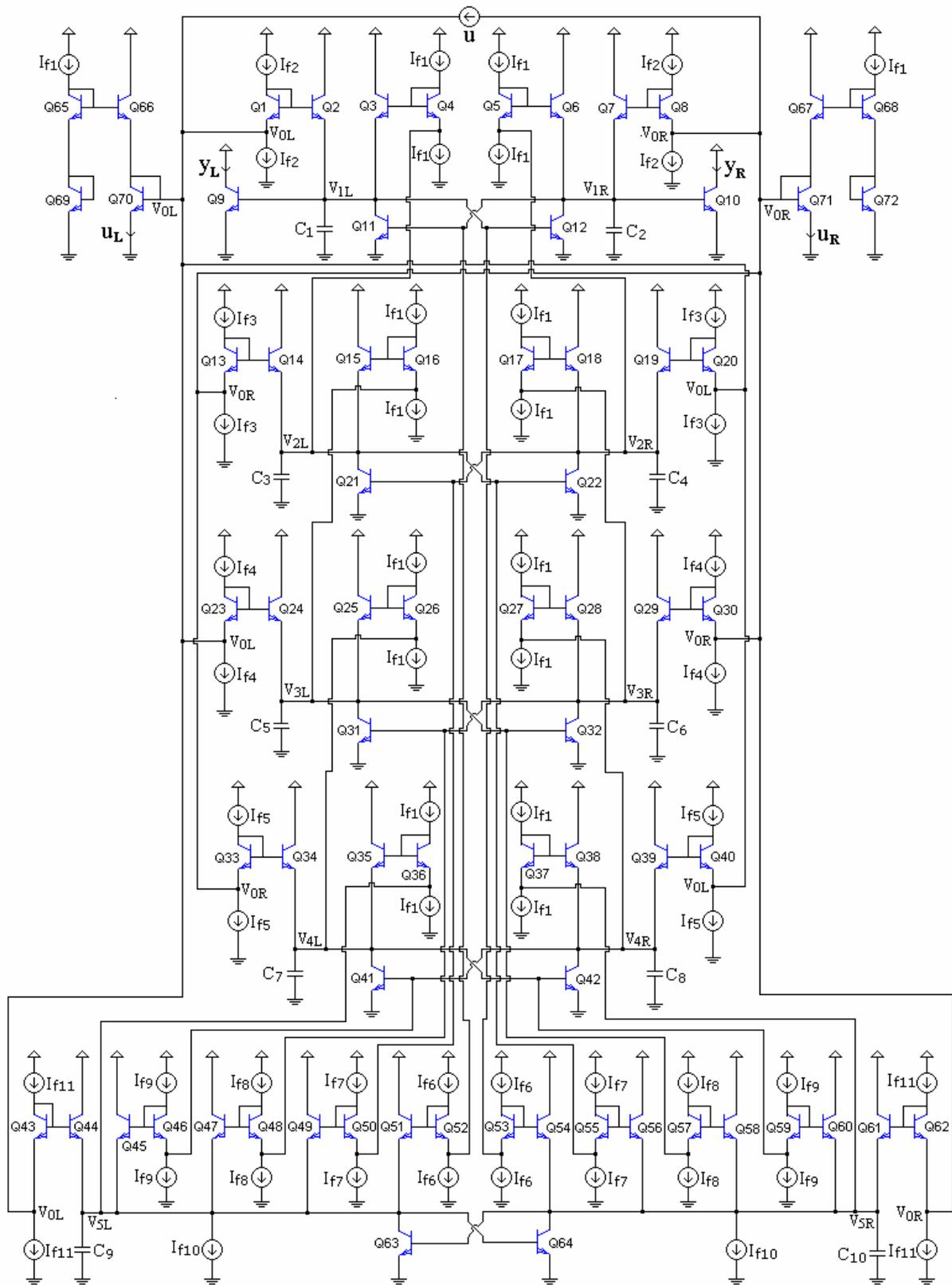
Figure 1. The current-mode 5th-order differential type class-AB log-domain elliptic lowpass filter
