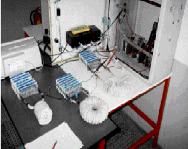
Fig. 2. At Left Front: Air-Core, Multiple Turns, Five Layers, Litz-Wire, Straight Cylindrical Inductor Design; At Right Front: Air-Core, Multiple Turns, Multiple Layers, Litz-Wire, Toroidal Inductor Design. Both Capable of Operating at 20 kHz, 500 V pk and 200 A pk .
