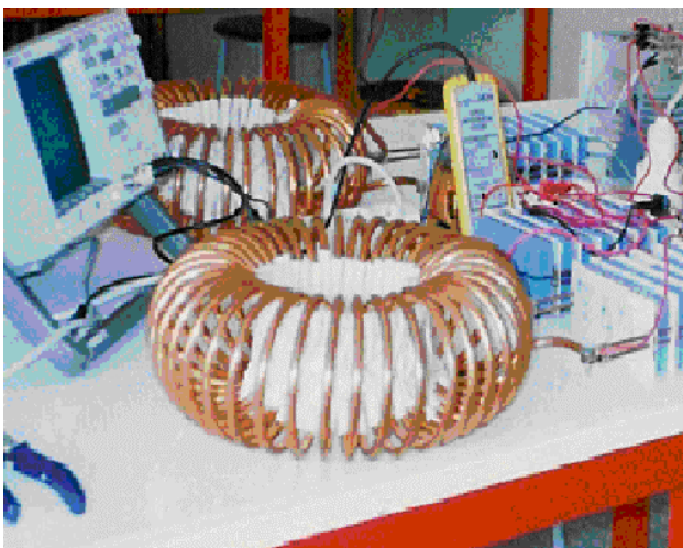
Fig. 5. A Toroidal Shaped Cylindrical Form Air-Core Inductor Design With Hollow Copper Wire Capable of Operating at 20 kHz, 500 V pk and 200 A pk .
