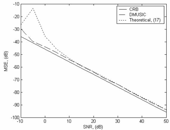
Figure 4. Theoretical and exact variances of DMUSIC and the CRB for frequency estimation of first complex damped sinusoid when  $\delta\omega = 1.5\Omega$ ,  $N\beta_1 = 1$ ,  $N\beta_2 = 0.01$ .
