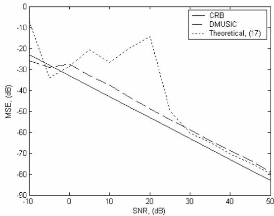
Figure 1. Theoretical and exact variances of DMUSIC and the CRB for frequency estimation of first complex damped sinusoid when  $\delta\omega = 0.5\Omega$ ,  $N\beta_1 = 0.01$ ,  $N\beta_2 = 0.01$ .
