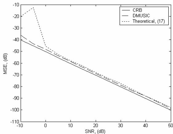
Figure 3. Theoretical and exact variances of DMUSIC and the CRB for frequency estimation of first complex damped sinusoid when  $\delta\omega = 1.5\Omega$ ,  $N\beta_1 = 0.01$ ,  $N\beta_2 = 0.01$ .
