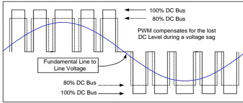
Fig. 1 PWM Voltage Boost Strategy during a voltage sag.
