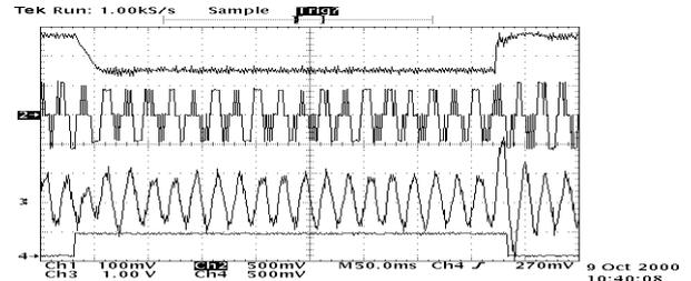
Fig. 9 Uncompensated case of 80% balanced voltage sag of 400ms duration; top: DC Link voltage, second: PWM voltage, third: motor current, bottom: trigger.
