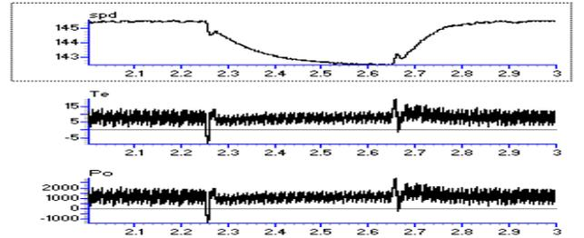
Fig. 3 Uncompensated Case: Predicted curves top: mechanical speed in rpm; middle: output torque in N-m; bottom: output power in watts.
