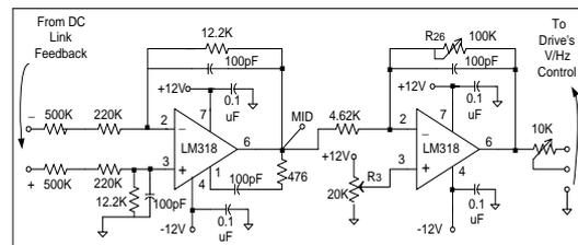
Fig. 7 Drives Volts/Hertz compensation circuit with a boost pulse.
