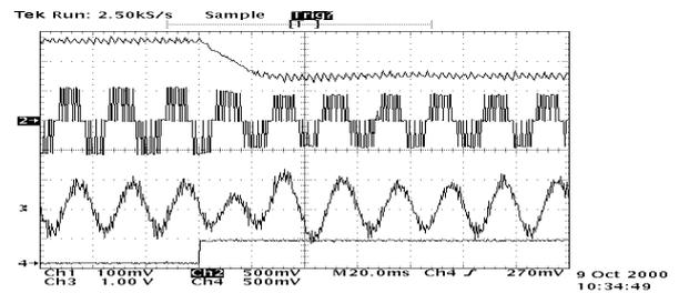
Fig. 10 Sag Initiation of the Fig. 9 uncompensated case of 80% balanced voltage sag of 400ms duration; top: DC Link voltage, second: PWM voltage, third: motor current, bottom: trigger.
