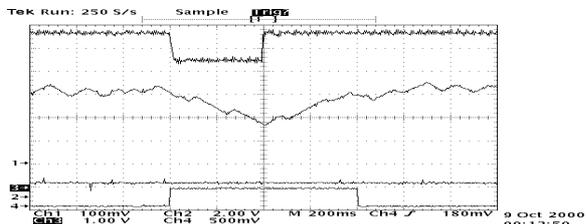
Fig. 8 Uncompensated case of 80% balanced voltage sag of 400ms duration; top: DC Link voltage, second: speed, third: boost voltage, bottom: trigger.
