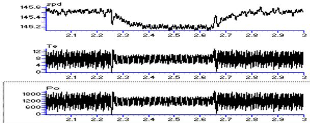
Fig. 5 Compensated Case: Predicted curves top: speed in rpm; middle: output torque in N-m; bottom: output power in watts.
