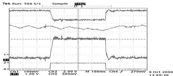
Fig. 12 Compensated case of 80% balanced voltage sag of 400ms duration; top: DC Link voltage, second: speed, third: boost voltage, bottom: trigger.
