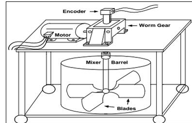
Fig. 6 Motor-Gear-Mixer Laboratory Prototype Setup.
