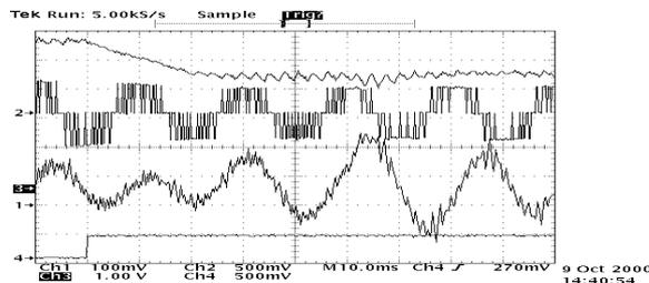
Fig. 13 Sag Initiation of the Fig. 12 compensated case of 80% balanced voltage sag of 400ms duration; top: DC Link voltage, second: PWM voltage, third: motor current, bottom: trigger.
