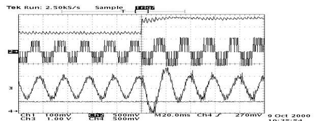
Fig. 11 Sag Recovery of the Fig. 9 uncompensated case of 80% balanced voltage sag of 400ms duration; top: DC Link voltage, second: PWM voltage, third: motor current, bottom: trigger.
