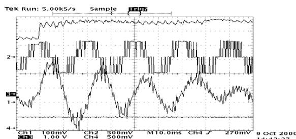
Fig. 14 Sag Recovery of the Fig. 12 compensated case of 80% balanced voltage sag of 400ms duration; top: DC Link voltage, second: PWM voltage, third: motor current, bottom: trigger.
