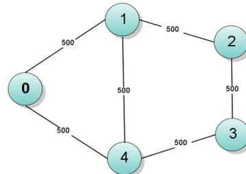
Fig. 3. Simple Mesh Topology
