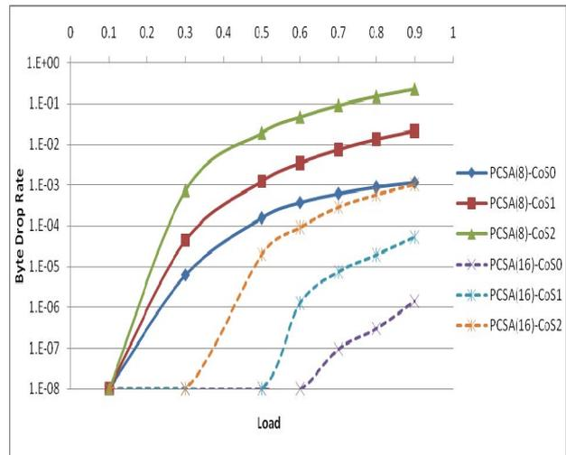
**Fig. 5.** Byte Drop Rates on NSFNET According to Number of Wavelengths
