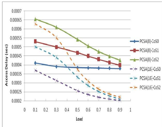
**Fig. 6.** Access Delay on NSFNET According to Number of Wavelengths
