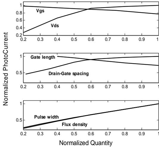
Figure 1. Effects of electrical bias, device geometry and optical input on output photocurrent. The output photocurrent in the figure is normalized to the maximum value in each case. The normalized x-axis corresponds to the following ranges: Vgs: 0 to -0.8 V, Vds: 1 to 5 V, gate length: 0.2 to 0.5  $\mu\text{m}$ , drain-gate spacing: 0.3 to 1.4  $\mu\text{m}$ , pulse width: 2 to 10 ps and flux density: 1 to  $20 \times 10^{21} \text{ cm}^{-2} \cdot \text{s}^{-1}$ .
