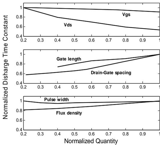
Figure 2. Effects of electrical bias, device geometry and optical input on output discharge time.
