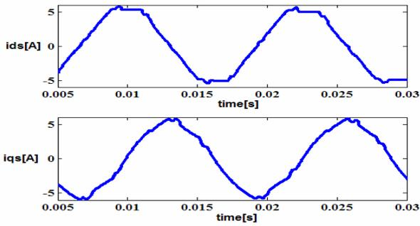
Figure 7. d-q stator current without MRAS based method.
