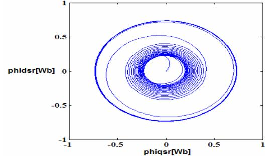
Figure 12. d-q rotor flux with MRAS based method.
