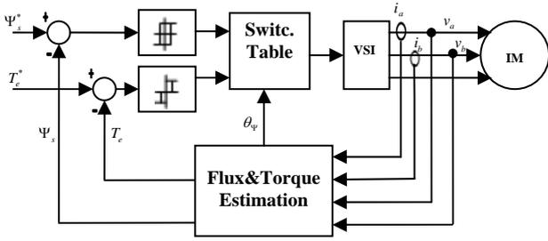
Figure 1. Basic DTC block diagram.
