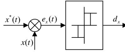
Figure 3. Three level hysteresis band control block diagram.
