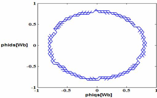
Figure 10. d-q stator flux with MRAS based method.
