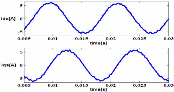
Figure 8. d-q stator current with MRAS based method.
