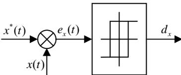
Figure 2. Two level hysteresis band control block diagram.
