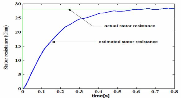
Figure 14. Stator resistance estimation at  $\omega_r = 20 \text{ rad/s}$
