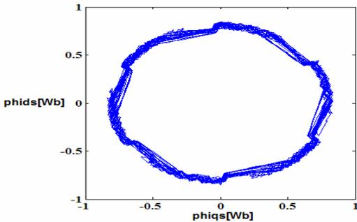
Figure 9. d-q stator flux without MRAS based method.
