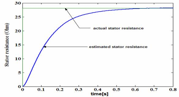
Figure 13. Stator resistance estimation at  $\omega_r = 314 \text{ rad/s}$
