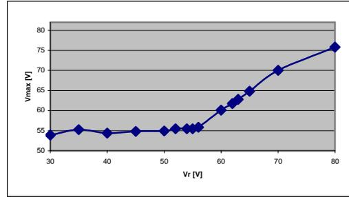
Figure 9: Maximum rail voltage vs voltage threshold of RPCDs ( $V_r$ ) for  $R_G = 0.1\Omega$ .
