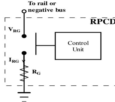
Figure 6: Rail Potential Control Device (RPCD)
