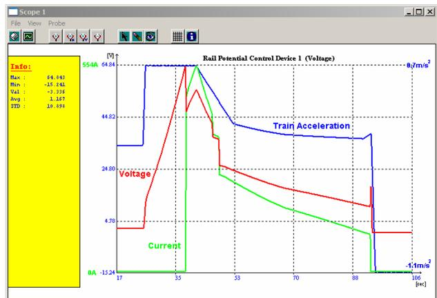
Figure 7: Change of voltage and current on RPCD1 and the acceleration graphics of the train.
