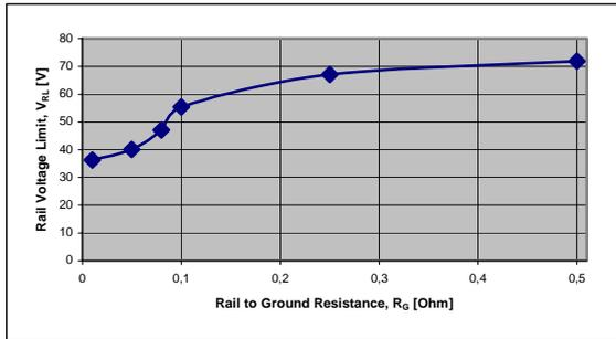
Figure 12: Rail voltage limit ( $V_{RL}$ ) vs rail to ground resistance ( $R_G$ ) for the test case considered.
