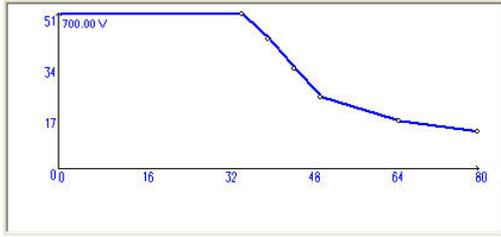
Figure 4. Tractive Effort (kN) – Speed (km/h)
