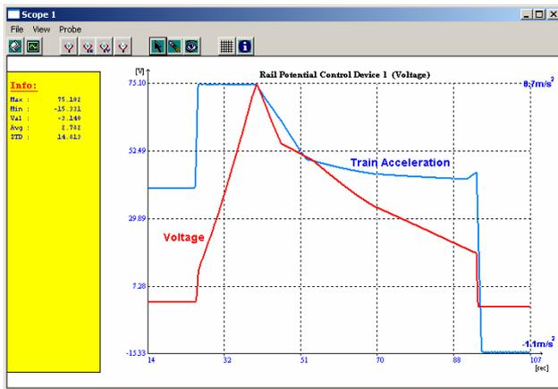
Figure 5: Change of train acceleration and rail voltage on the first passenger station without the use of RPCDs.
