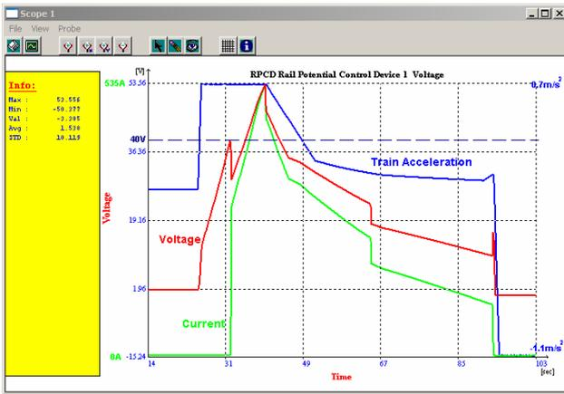
Figure 8: Change of voltage and current on RPCD1 and the acceleration graphics of the train for  $V_r = 40$  V.
