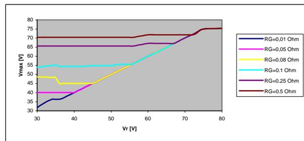
Figure 11: Maximum rail voltages for different settings of  $V_r$  and  $R_G$ .
