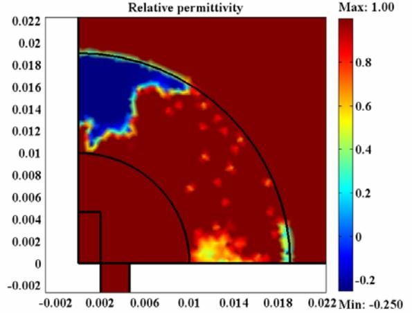
Figure 2. Relative permeability distribution and its corresponding values for a metamaterial shell-based electrically small antenna obtained with topology optimization.
