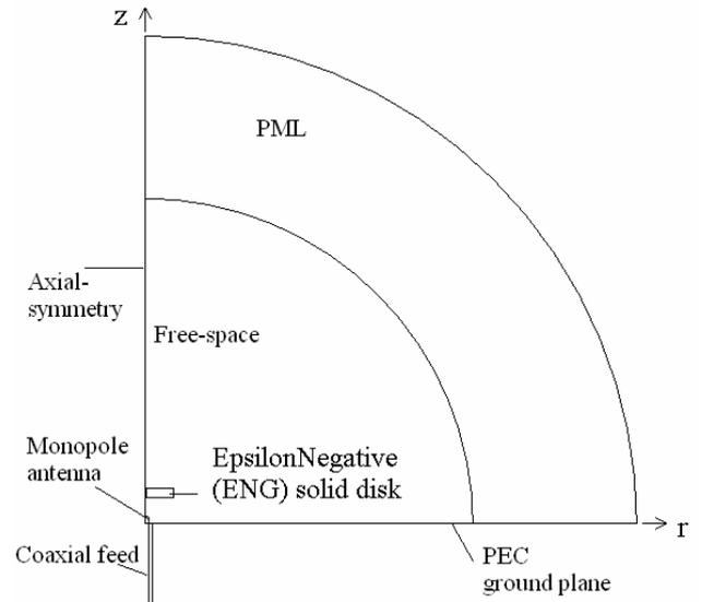
Figure 3. A finite element model of the coaxially-fed copper monopole-ENG solid disk antenna system
