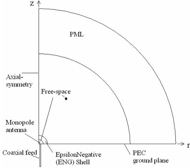
Figure 1. A finite element model of the coaxially-fed copper monopole-ENG shell antenna system
