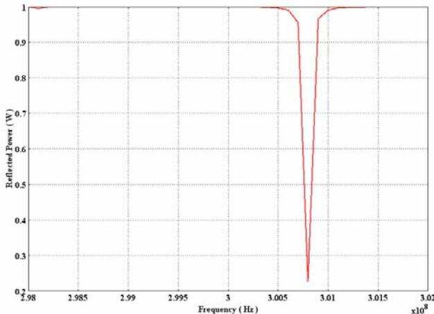
Figure 4. The frequency response of the reflected power,  $|S_{11}|^2$ , for the proposed metamaterial solid disk-based electrically small antenna given in Fig. 3.
