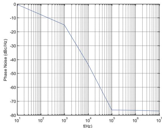
Fig. 11. Measured phase noise of the realized DRO
