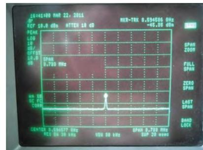
**Fig. 9.** Power spectrum of the second harmonic of the oscillation frequency.
