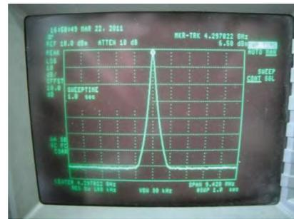
**Fig. 8.** Output spectrum of the dielectric resonator oscillator
