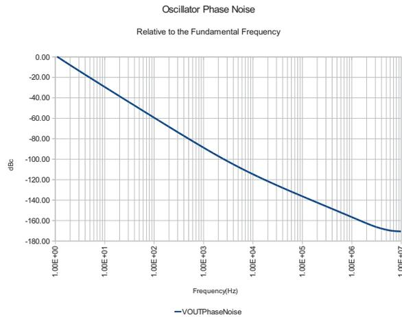
**Fig. 6.** Harmonic balance simulation results - phase noise relative to the fundamental frequency
