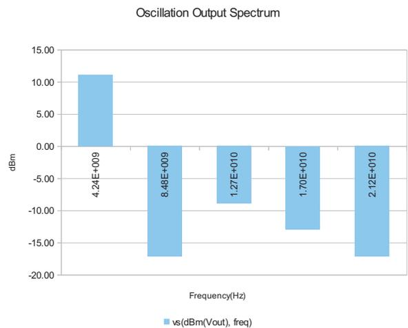
Fig. 5. Harmonic balance simulation results - spectrum components
