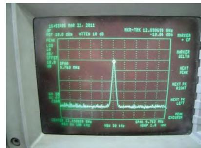
**Fig. 10.** Power spectrum of the third harmonic of the oscillation frequency.
