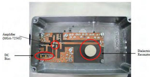
**Fig. 7.** Picture of the printed circuit board
