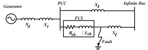
**Fig. 2.** The power system with the proposed FCL
