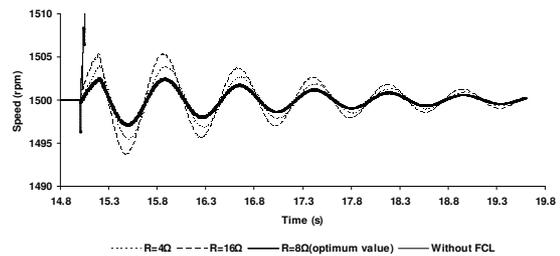
**Fig. 8.** Rotor speed oscillations of the generator
