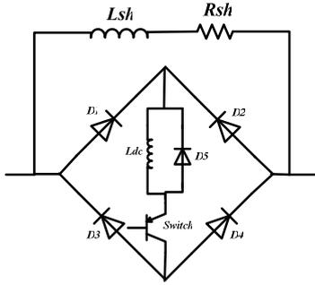
**Fig. 1.** Power circuit topology of the proposed FCL
